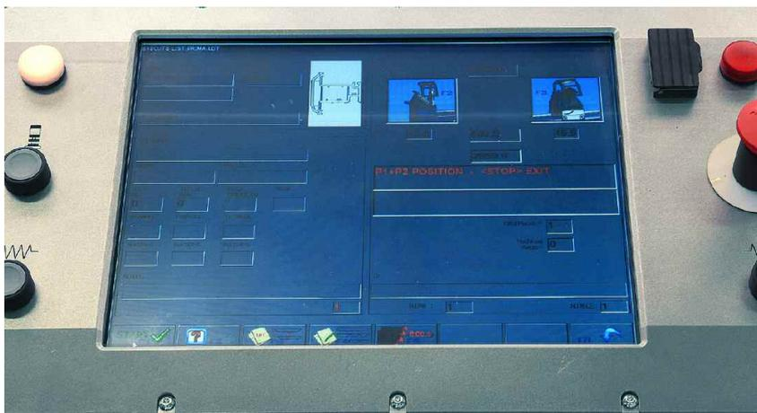
Besides these advantages connected to the choice of the operative system, the 500 TS presents a large sized touch screen display with intuitive graphics which also gives the operator an easy and fast use of the machine in semiautomatic. A help on line in HTML format also allows access to all the technical information on the machine (electrical and pneumatic diagrams) and to that information for the solution of possible problems on the same.
