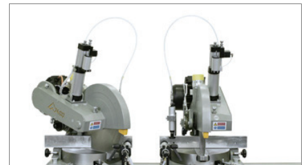
Rotation of the moving cutting heads
