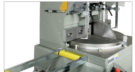
Blade and roller conveyor 02
